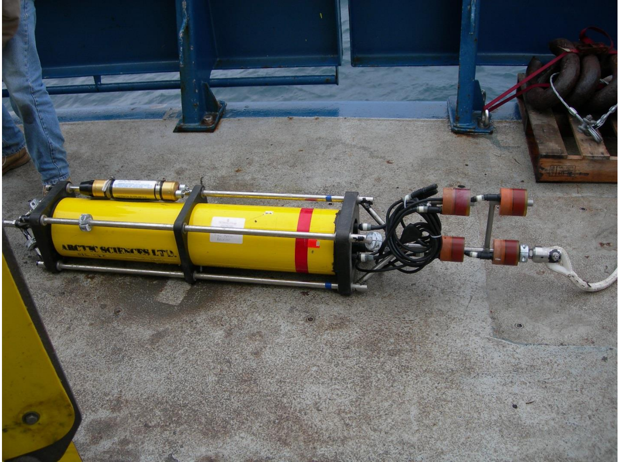
Figure 41. This is the receiver portion of the ASF (acoustic sensor), it is shown to highlight the importance of being delicate as we deploy the mooring line and fragile instrument components. This instrument and frame is 6.43 ft long.
