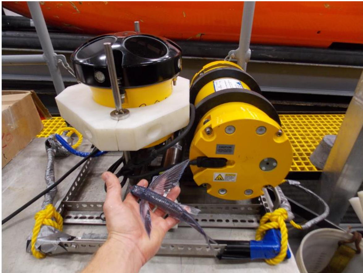
Figure 4. Unit 3 fully assembled. There is a lifting rope on each side of the frame, with a loop built in for grabbing with the ROV hand. The lifting ropes are still installed.
