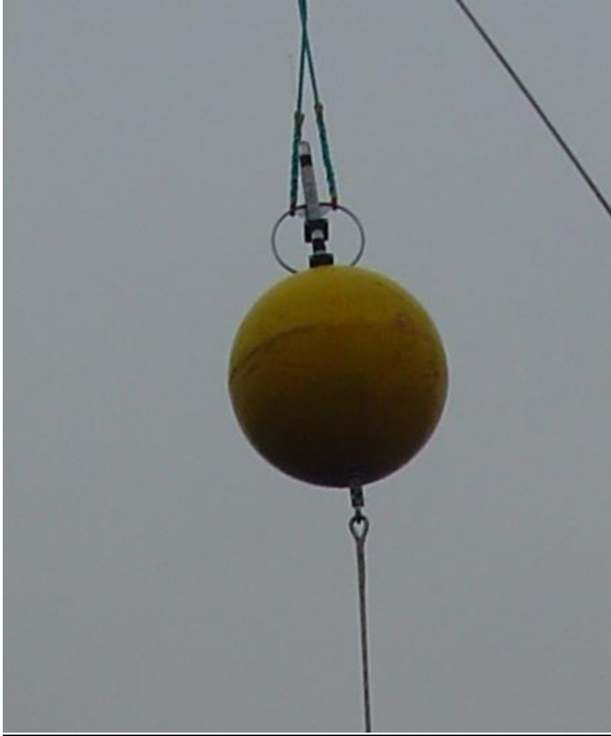
Figure 10. The buoy for Unit 5 and 6. There is a circular lifting bail on top of the buoy, which should serve as our lifting point. In this image there is a light beacon that is not be present on this deployment.
