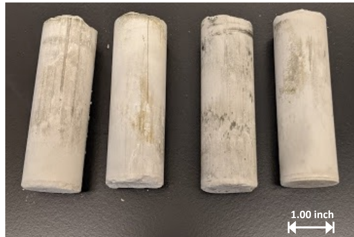
Fig 11. Trial Flexcem cement cores Ready for testing
