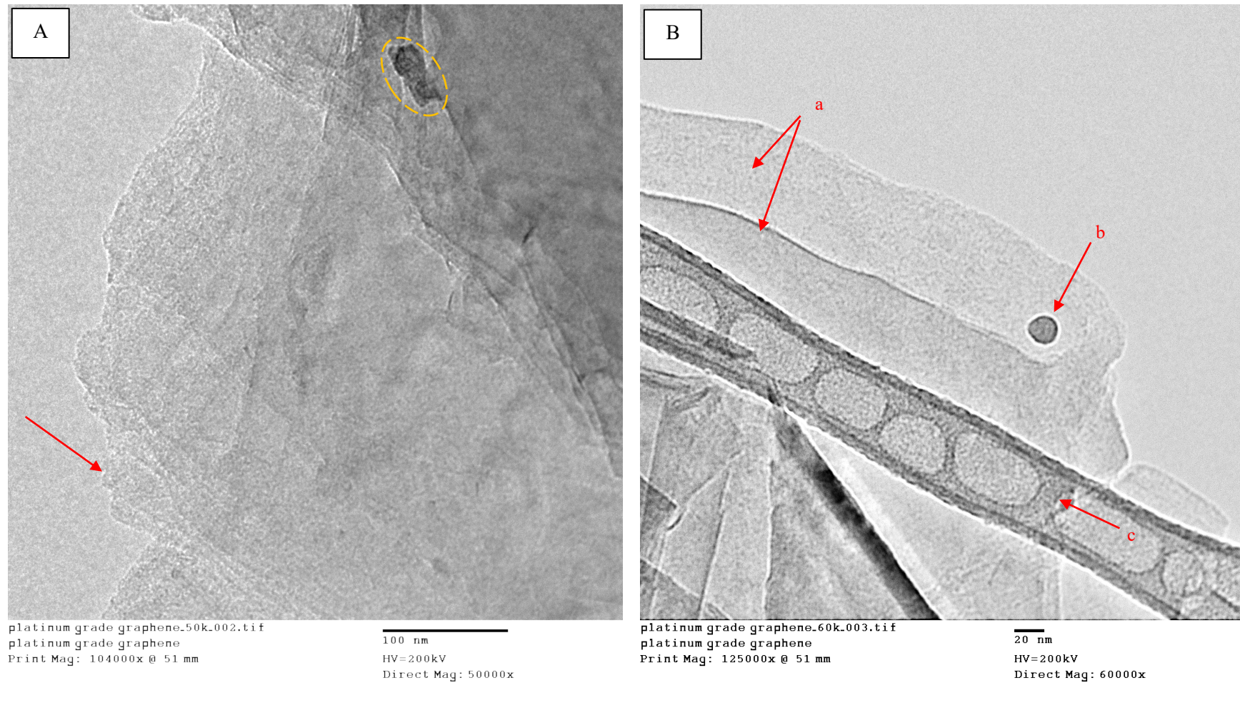
Figure 3: A) Multiple layers of nanosheets are stacked on each other orderly. Defined lines are an indication of a platelet edge and darkening color indicating thicker sections. B) High magnification image at the edge of graphene cluster.
