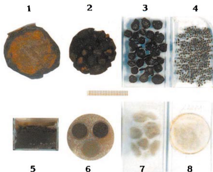
Figure 4-1. Modes of sample preparation: (1) single clinker, impregnated with epoxy resin, cut, and polished; (2) crushed clinker fragments, encapsulated and impregnated with epoxy, cut, and polished; (3) whole clinkers impregnated with epoxy and mounted on a thin film of epoxy on a glass microscope slide, cut and polished; (4) millimeter-size crushed clinkers, embedded in epoxy, ground, and polished; (5) cement, size graded by sedimentation in an alcohol-mineral spirits mixture in a glass vial, dried, impregnated with epoxy, cut, and polished; (6) drilled holes in an epoxy plug, filled individually with cement (a) extracted with a potassium hydroxide-sugar solution, (b) extracted with maleic acid, and (c) unextracted—the plug has been cut and polished; (7) thin section of whole clinkers; section thickness is approximately 22 \mu m; (8) crushed clinker, 45- to 75- \mu m fraction, in Hyrax, for determination of the kiln parameters with the Ono Method. Scale divisions in mm. (S#A7094)
